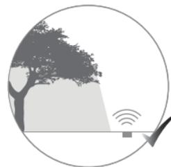
For maximum efficiency we recommend you to Install **Brick** solar lamp where it can get direct sunshine, free from cover or shade.
